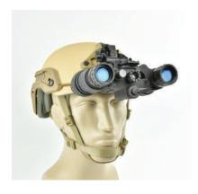
The BNVDG can be used as a monocular by choosing which side you want to use as your night vision eye and rotate the other side/arm of the binocular up and out of the way. Each arm is tight enough so that the rotated arm will not fall down, but stay in its user adjusted position. To use as a binocular, rotate both sides down or when night vision is no longer needed, shut off and rotate both sides up and out of the way.
