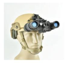
The BNVDG can be used as a monocular by choosing which side you want to use as your night vision eye and rotate the other side/arm of the binocular up and out of the way. Each arm is tight enough so that the rotated arm will not fall down, but stay in its user adjusted position. To use as a binocular, rotate both sides down or when night vision is no longer needed, shut off and rotate both sides up and out of the way.
